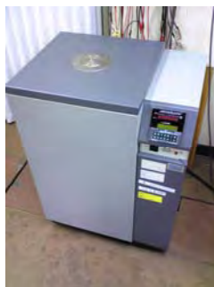
電気炉 :Hart 9115 Control panel: Bob S619p
